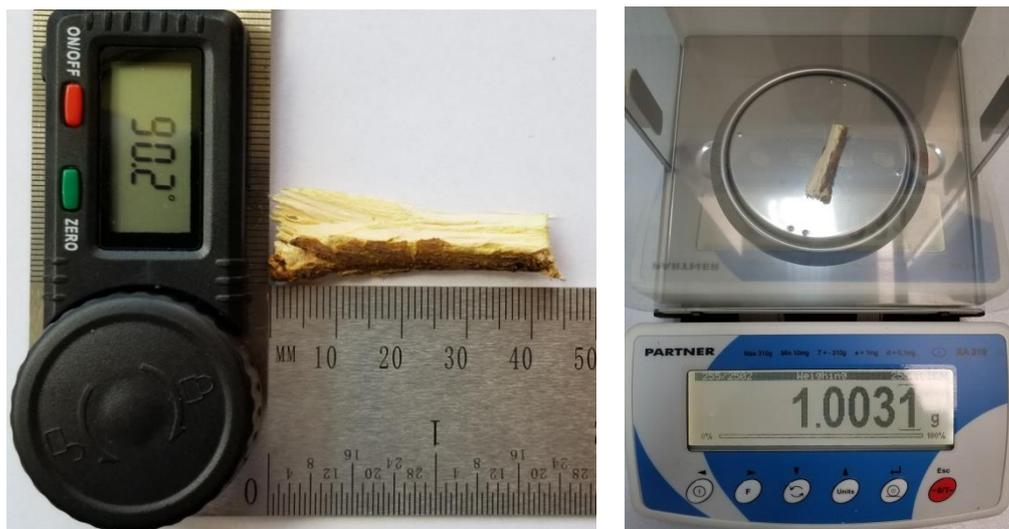
**Fig. 4 - Biomass particle dimensions and mass**
