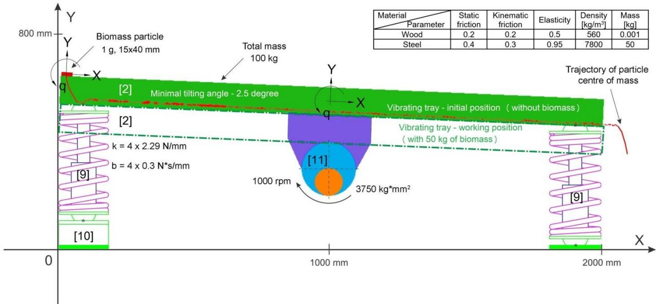
**Fig. 3- Physical simulation model of the dryer**
