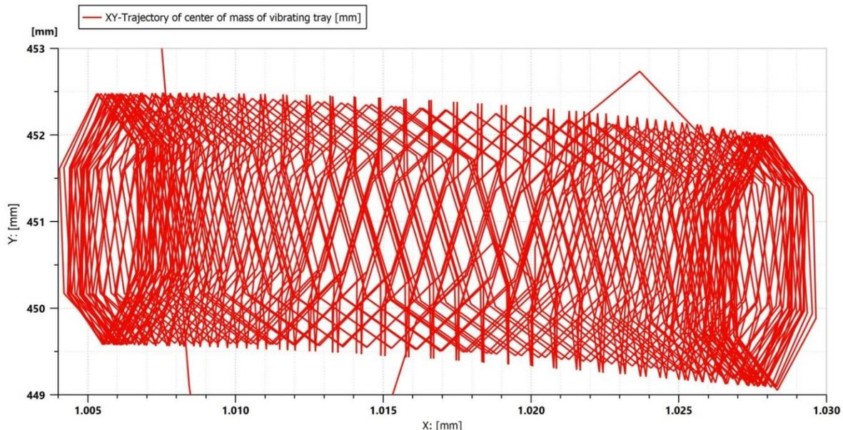
Fig. 6 - XY-Trajectory of centre of vibrating tray mass
