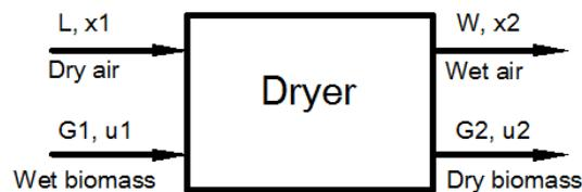
**Fig. 1- Block diagram of the artificial drying process**
