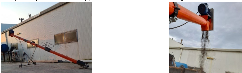
Fig. 6 - Handling of chopped biomass (chopped branches, with maximum granulation of 35 mm)
