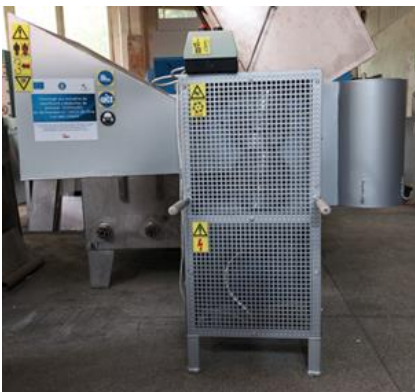
Fig. 3. Chopper driven with electric engine of 2.2 kW
