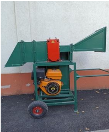
Fig. 2. Chopper driven with thermal engine of 13 CP
