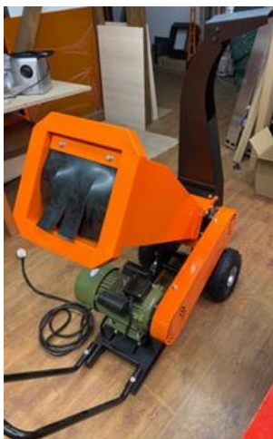
Fig. 4. Shredder driven with electric engine of 4 kW
