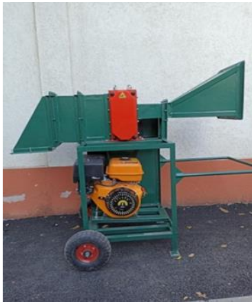
Fig. 2. Chopper driven with thermal engine of 13 CP
