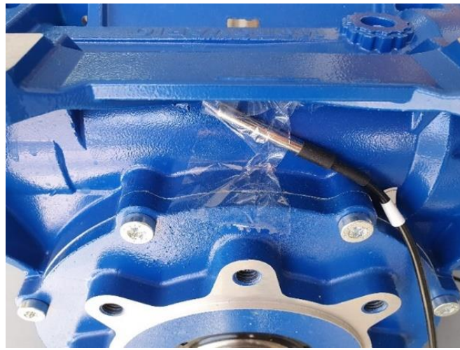
Fig. 7. OneWire IP67 temperature sensor
