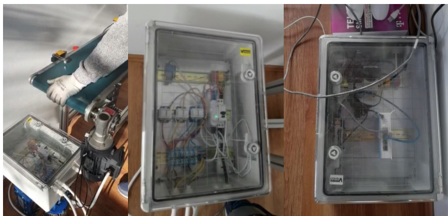
Fig. 8 – Mounting of the automatic control module
