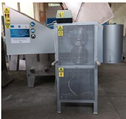
Fig. 3. Chopper driven with electric engine of 2.2 kW
