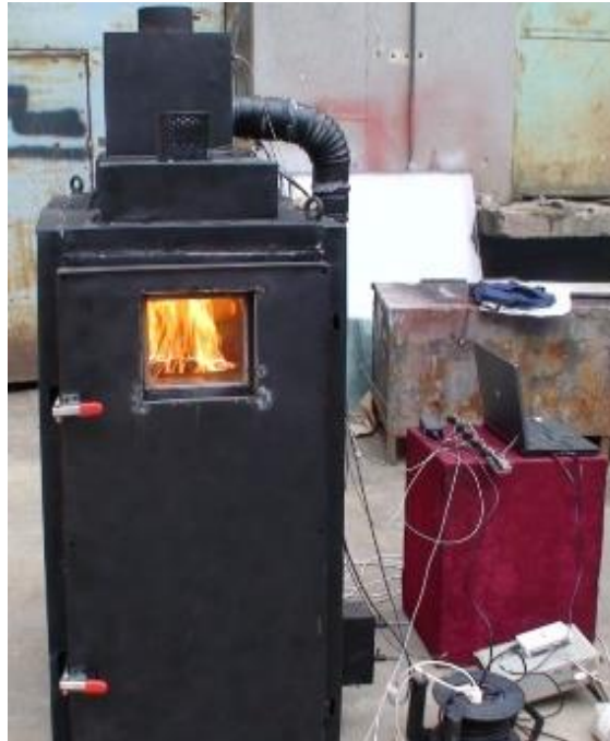
Fig. 5. PLC device equipping the TLUD heat generator
