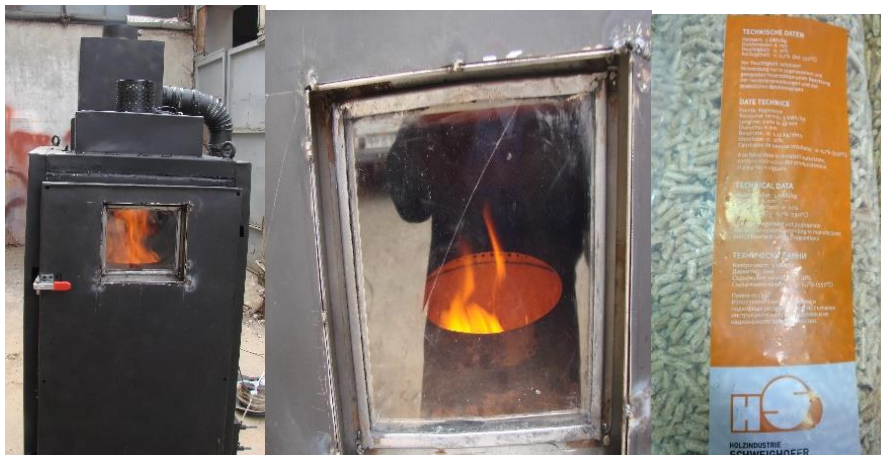
Fig. 3. Experimental model of a TLUD gasifier
