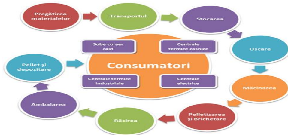
Fig. 1. The technological flow of pellet production and distribution, [8]
