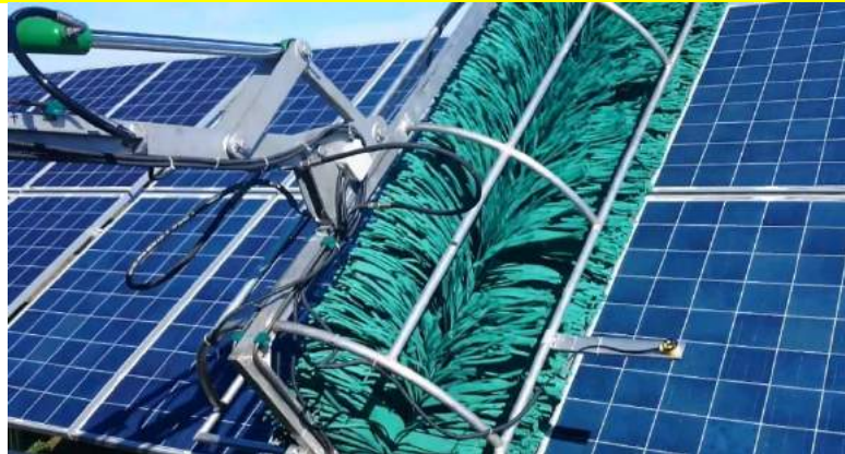
Figure 2: Folding mechanism of brush driven with hydraulic cylinder
